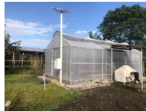
Hybrid solar dryer for coffee in Uganda
